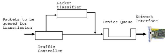
**FIGURE 1:** *Flow of data packets through the traffic controller*
